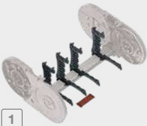
1 Insert cables, open dividers and insert first height separator
