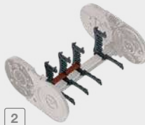
2 Insert additional cables, insert height separators
