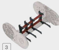
3 Insert cables, complete height separators
